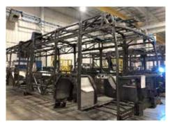
The frame of a new GoWest bus is assembled at a factory in Alabama.
