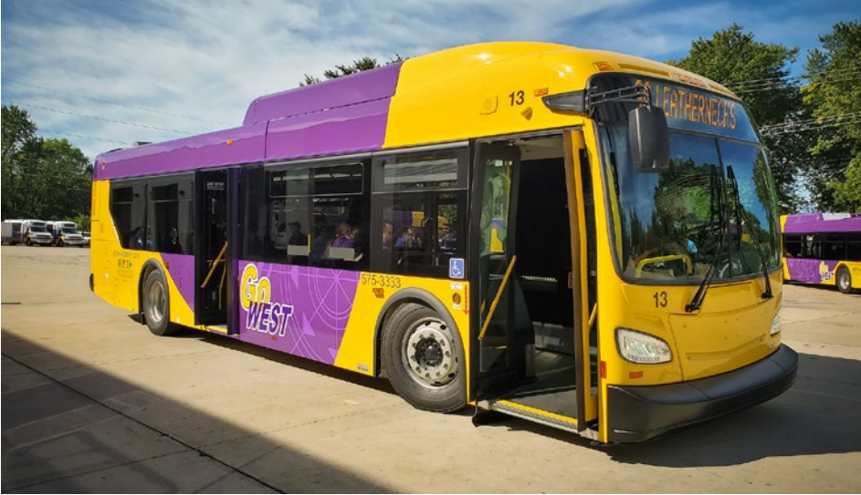
One of McDonough County Public Transportation's five new 35-foot, 24,000-pound New Flyer Excelsior Clean Diesel buses is displayed at a media event on September 13, 2019.
